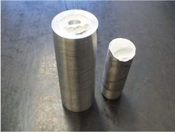
Fig. 11: Fractured aluminium spigot taken from stainless steel stanchion (TEST#1).
