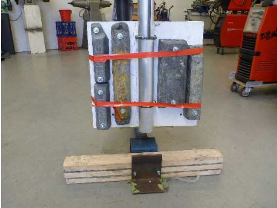
Fig. 9: 100kg lead weights on back face.
