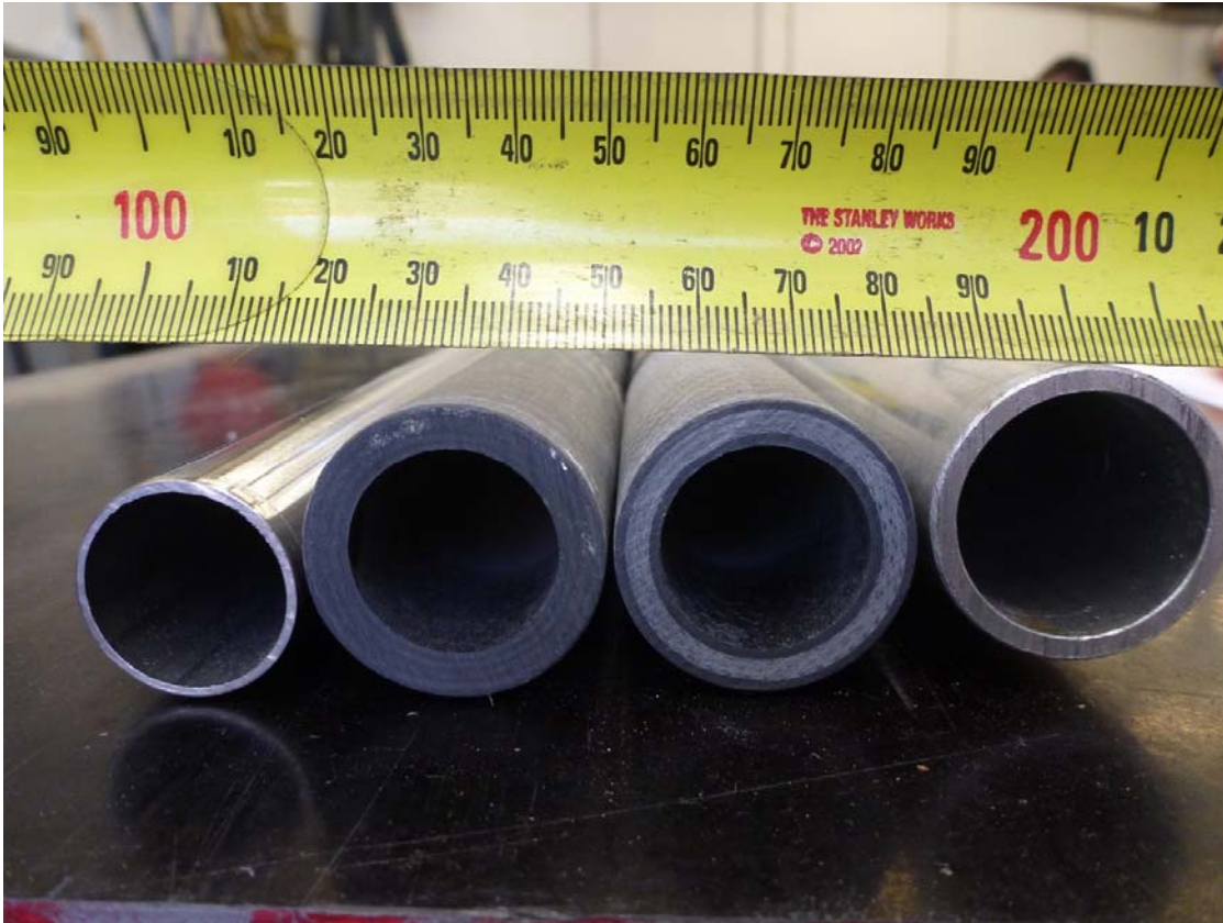
Fig. 7: Left to right - Stainless steel \phi 25 \times 1.6 ; carbon fibre \phi 29.6 \times 5.0 ; carbon fibre/E-glass \phi 32 \times 5 ; aluminium \phi 31.5 \times 2.5
